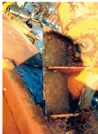
Fig. 56. Fall of the hanging stage of autohydraulic hoist VS-22 on the roof of the one-storey building: a — drawing of the accident; b — the area where the bracket torn of the fastening of the hydraulic cylinder
