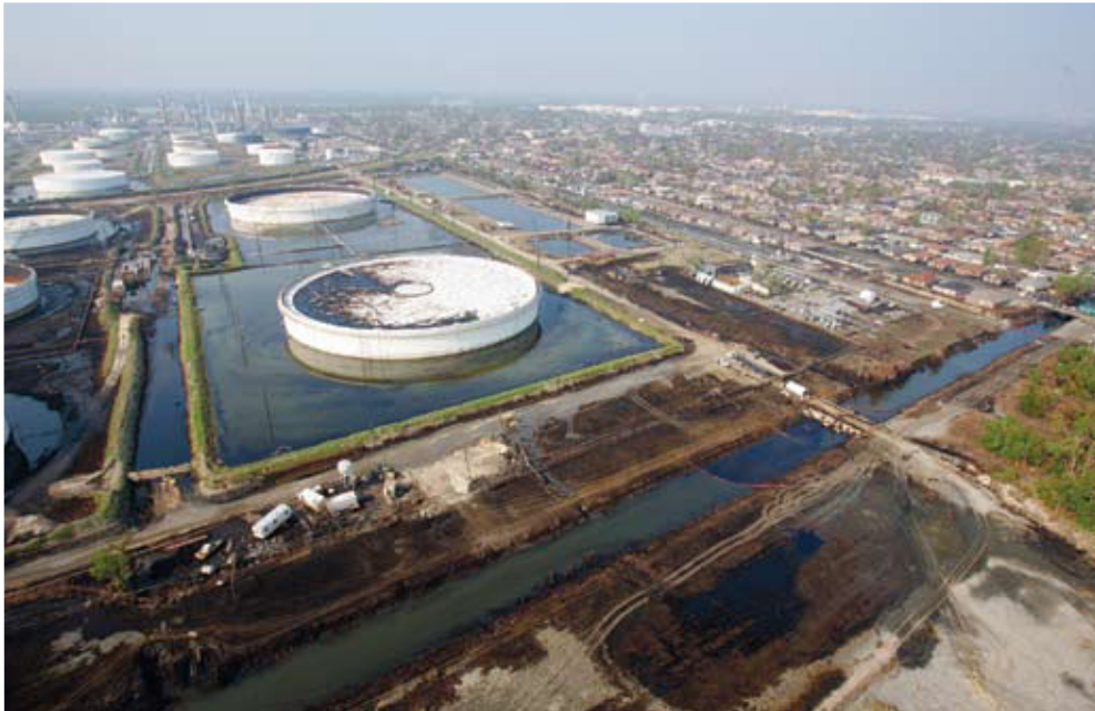
Figure 2.2 Flooded Petroleum Storage Tank Farm
